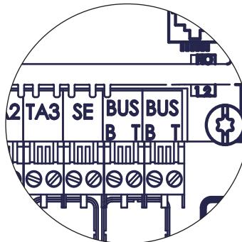
3) Make the electrical connections between the "BUS" terminal block on the boiler (B and T) and one of the two "BUS" terminal blocks on the module (B and T).
