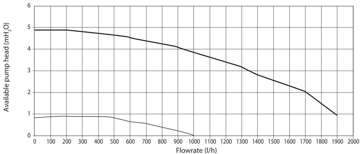
Zones 2 & 3 available pump head mixing valve, lever in lowered position (A → AB)
